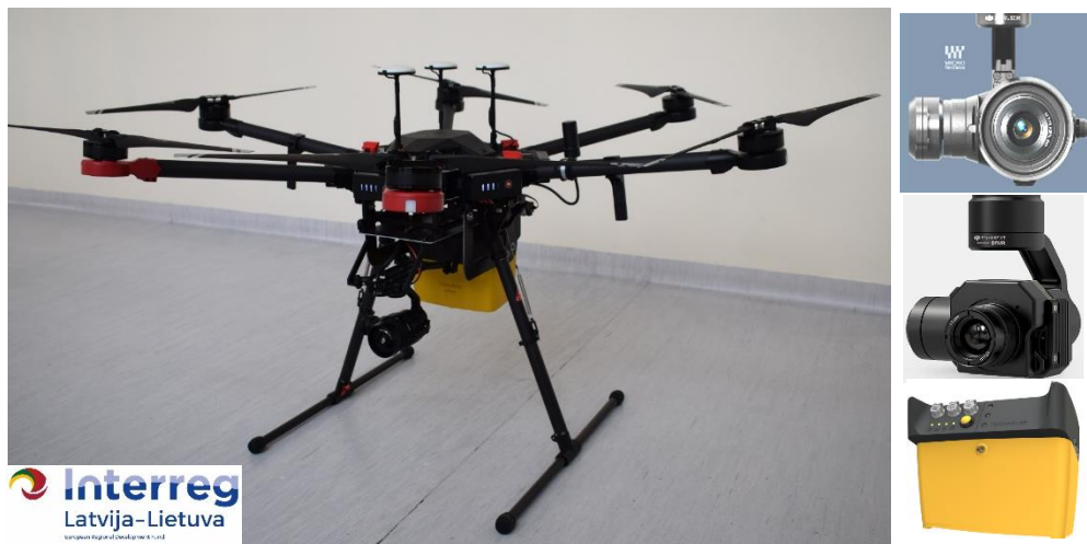
Fig. 1. UAV - Photogrammetry system available at KVK: Drone DJI MATRICE 600 PRO , gimbal camera DJI Zenmuse X5 , gimbal thermal camera DJI Zenmuse XT , laser scanner (LiDAR) Mapper Lite 2 , GPNS Source: created by authors
