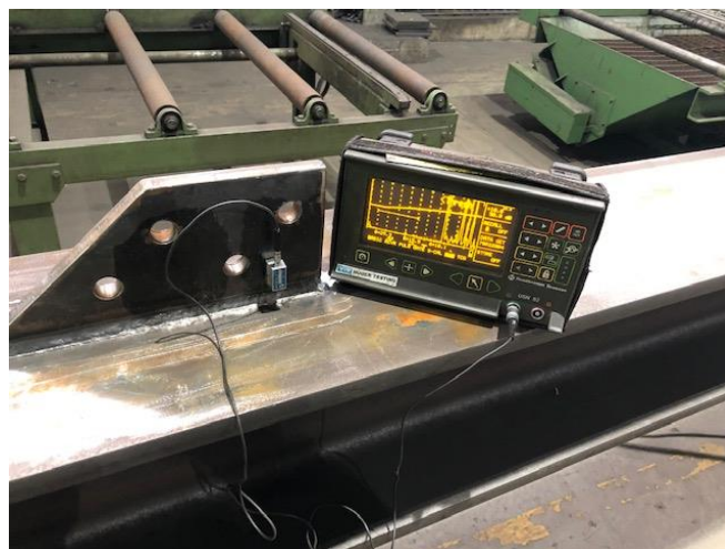
Fig. 1 Ultrasound scanner USM 25 with signal converters MWB 70-4 for checking the full penetration seams
