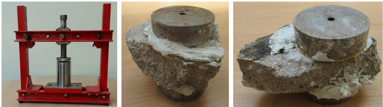
Fig. 2. Specimen centering equipment and irregularly shaped specimens with concave dies
