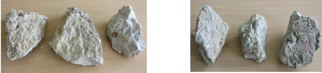
Fig. 1. Irregularly shaped concrete pieces for specimens
